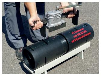
Fitting the manual insertion tool
